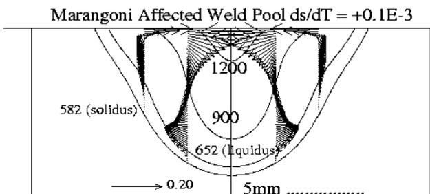
Figure 5b: Positive: Temperature and flow fields [8]
