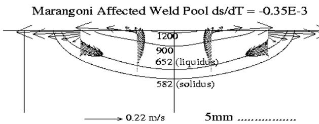
Figure 4a: Negative: Temperature and flow fields
