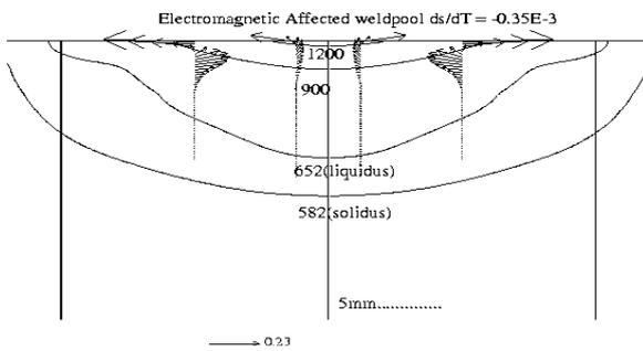
Figure 8a: Negative surface tension and Lorentz forces.
