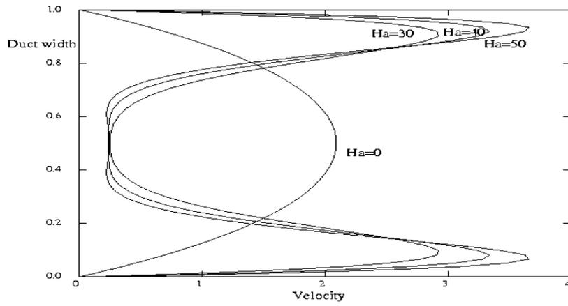
Figure 7: Profiles of Magneto hydrodynamic duct flow
