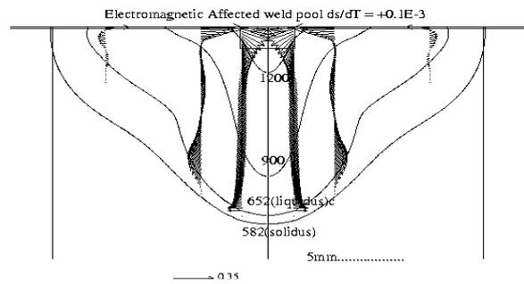
Figure: 8b: Positive surface tension and Lorentz forces.
