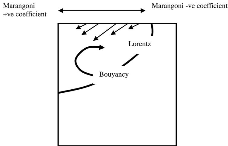
Figure 9: Relative direction of the affecting Forces
